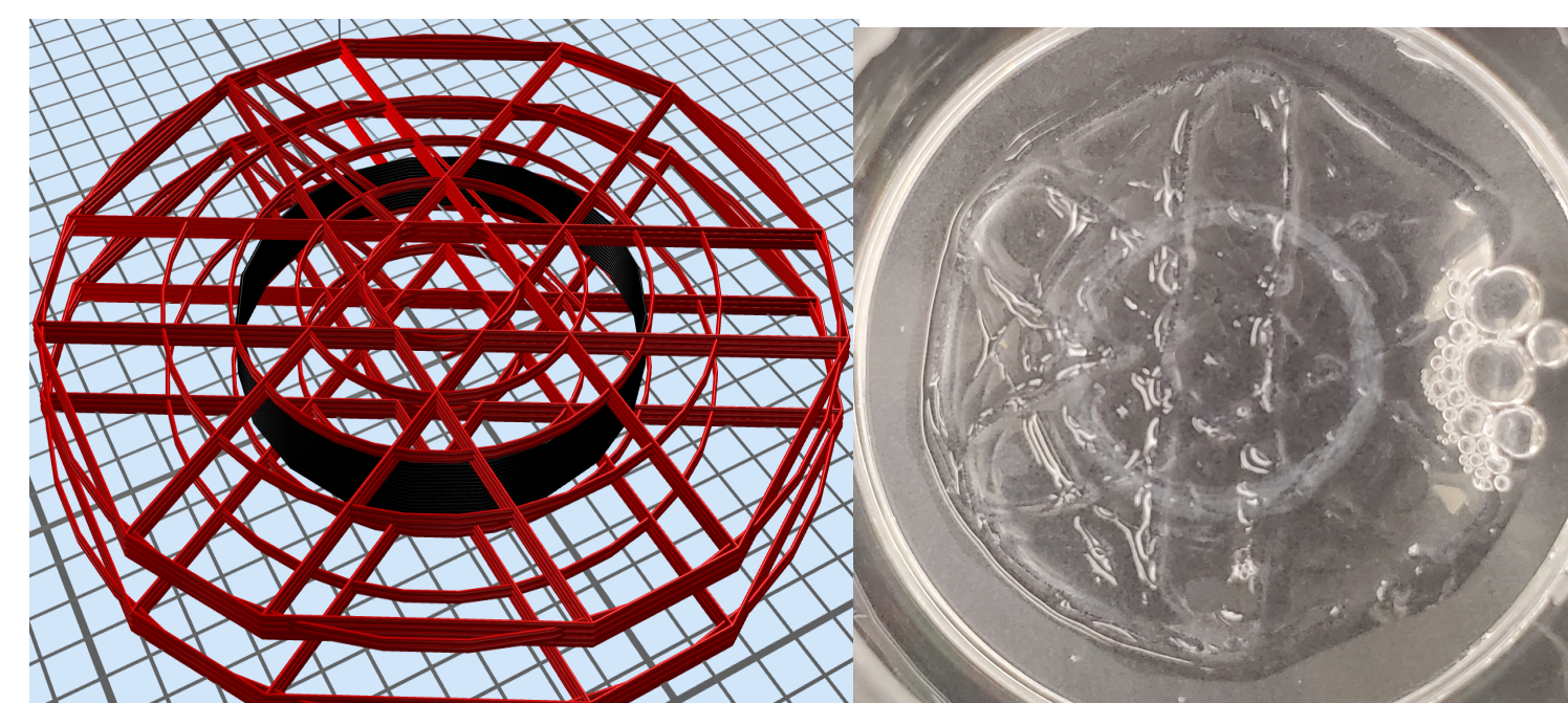
Figure 1. Visual depiction of the spiderweb design and printed construct. ASM ring constrained between 6 layers of acellular ink above and below.
