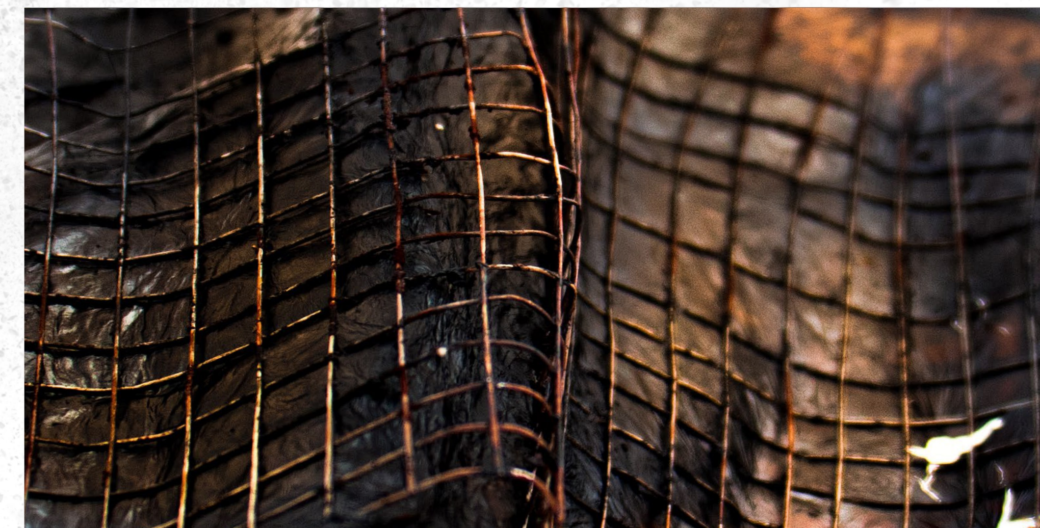
Fig 4. Oxidized bacterial cellulose sheet dried on a steel galvanized mesh
