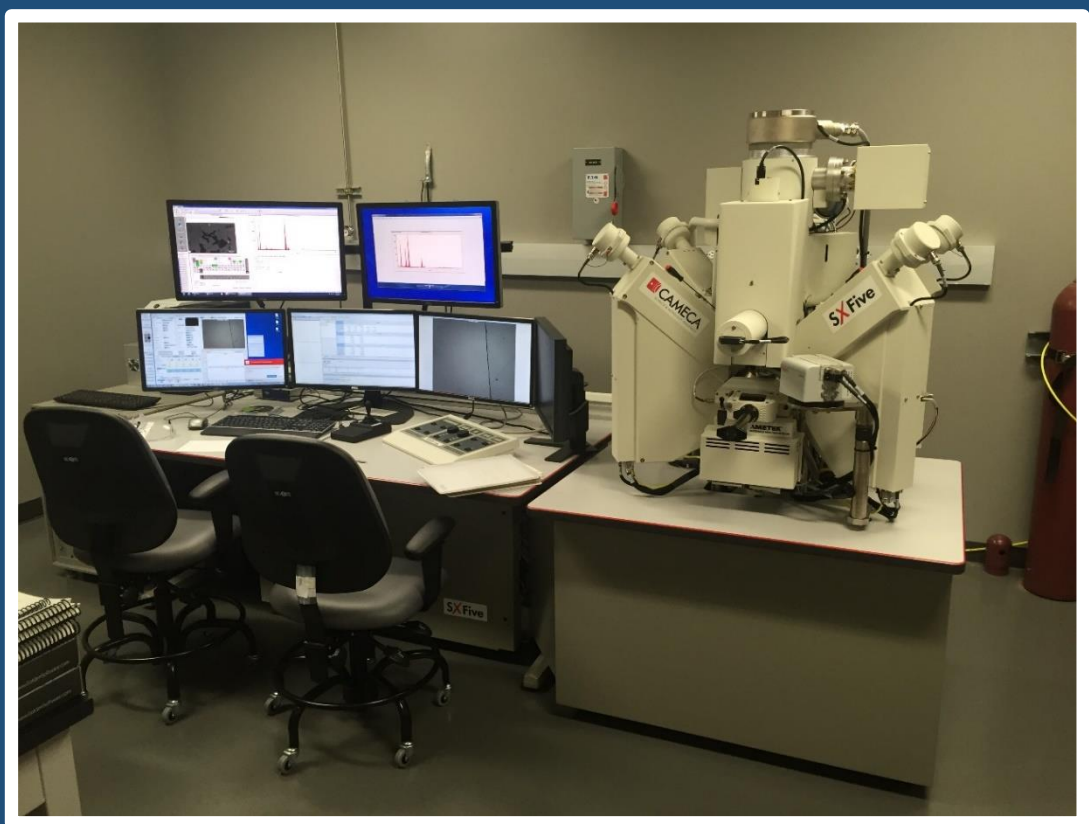
Figure 9: EPMA used for compositional analyses of pyrite and sphalerite ( https://mcf.tamu.edu/instruments/electron-microprobe/ )
