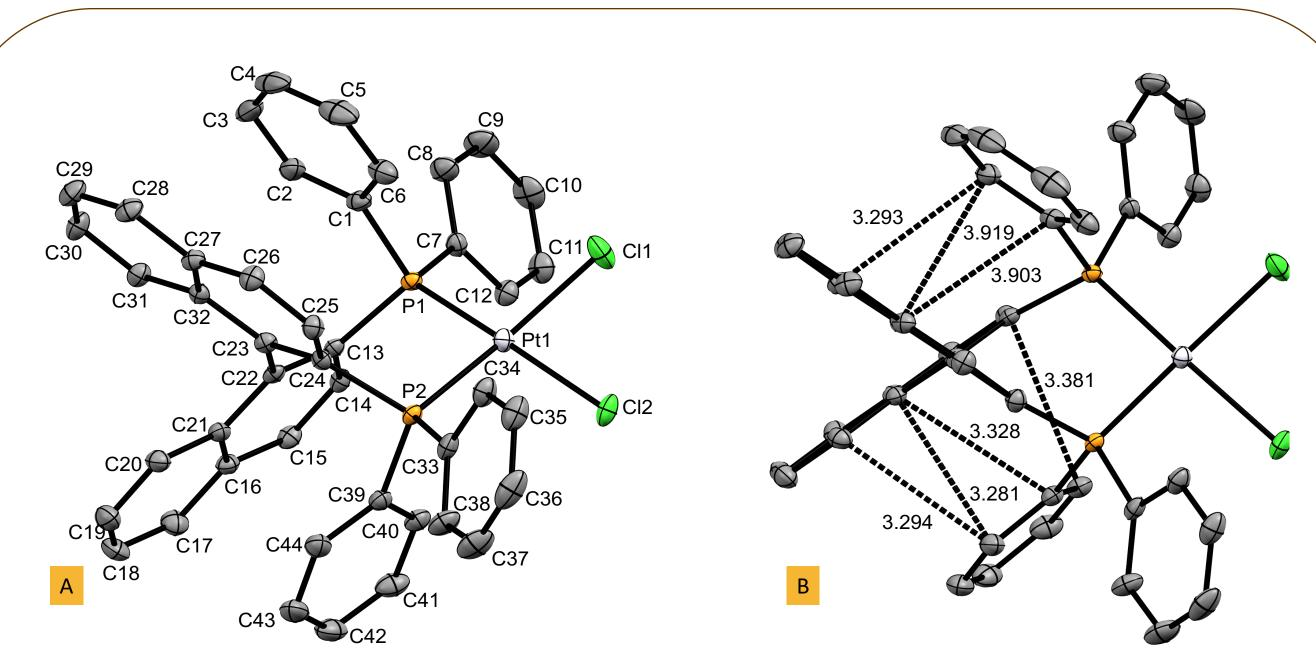
**Figure 4.** Crystal structure of (BINAP)PtCl<sub>2</sub> showing (A) atom labels of the R enantiomer (B) close contacts. Phosphorous atoms of BINAP are in yellow, and the Platinum atom is in white. Hydrogen atoms and solvent molecules are omitted for clarity.
