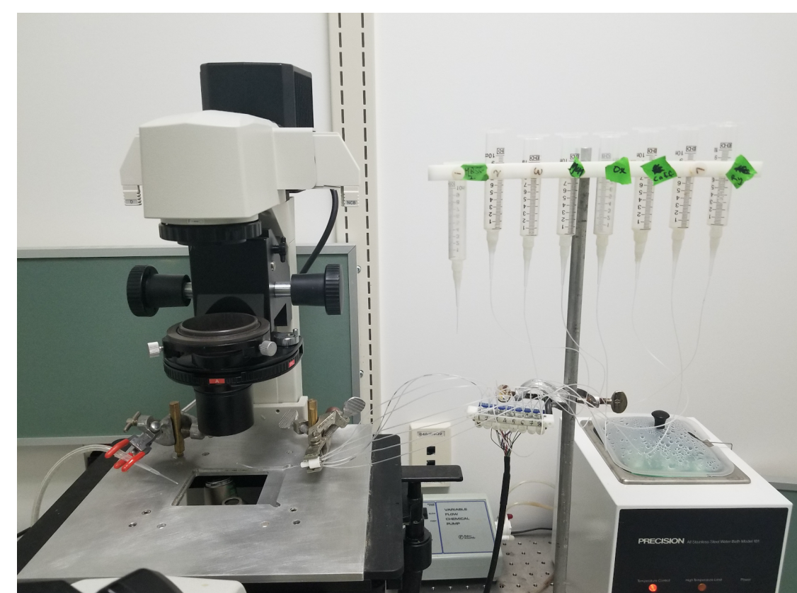
Figure 2. Set-up of experiment showing the phase-contrast microscope and the solenoid valve system for controlling solution flow
