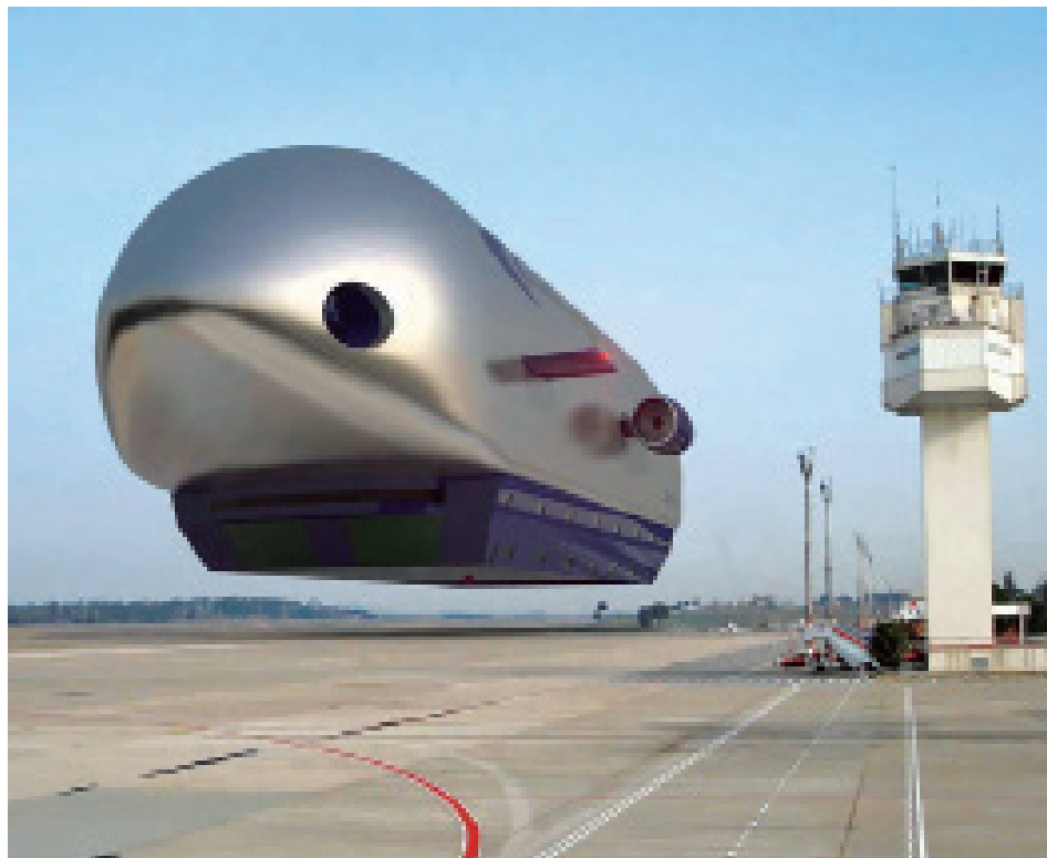
A rendering of a Varialift 'monocoque' all-aluminum airship. Airships are said to product 80%-90% less carbon emissions than conventional aircrafts, and, if used to transport cargo into Canada's northern region, would help bring business to the trucking industry.
